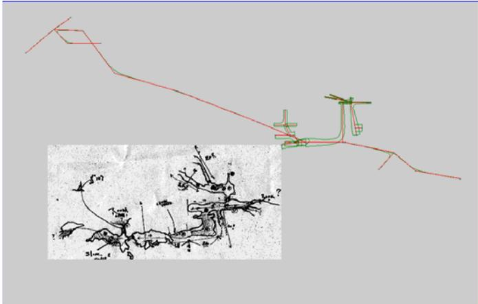
Mike Eaton's sketch map of No-Bottom Pond Cave, alongside a Compass line plot with LRUD-generated passage dimensions. Cave survey using Brunton Compass and tape. Some dimension data estimated from the sketch. Surface survey line plot connects surface sinks and openings.
