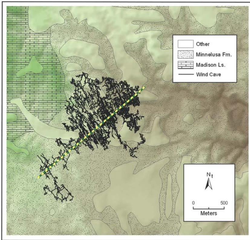
**Figure 2. Relationship of the Madison Limestone outcrops to the Wind Cave survey. The major trend of the cave is marked with a yellow and green striped line. The Minnelusa Formation lies directly above the Madison limestone. This illustration was created by combining a shaded relief DEM, geology layer, and survey lineplot.**
