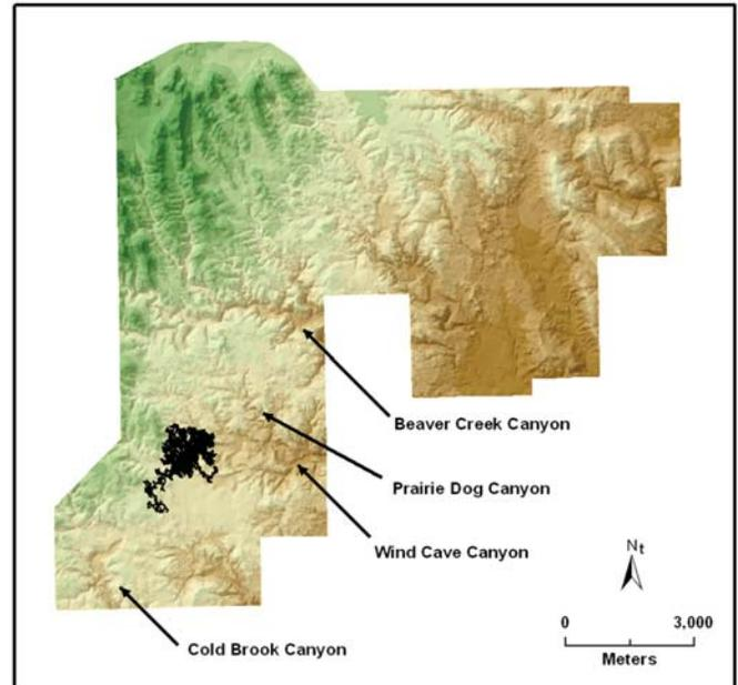
**Figure 1. Location of Wind Cave within Wind Cave National Park. The Wind Cave survey lineplot (black) was generated using COMPASS software and imported to GIS format and georeferenced using the CaveTools extension for ArcView GIS. The cave data are plotted atop a digital elevation model (DEM), which has been shaded showing higher elevations in green and lower elevations in brown.**
