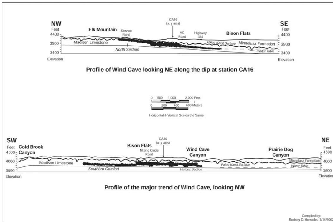
**Figure 3.** Profiles of Wind Cave along the major trends of the cave, showing the relationship of surveyed passages with the structural geology. Station CA16 was chosen because of its location at the intersection of the two major trends of cavern development. This illustration was compiled from the Wind Cave National Park and Vicinity 20-foot contour map, COMPASS data, geology maps, cave radio location data, and GIS hydrography layers.
