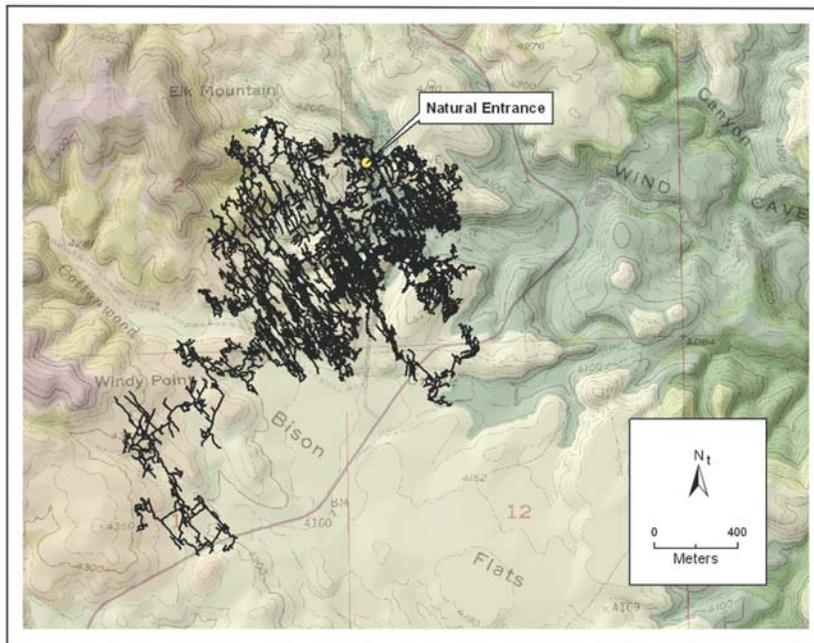
**Figure 5. Wind Cave entrance location and surface relief. A DEM was used to create a surface upon which the Wind Cave USGS digital raster graphic (DRG) was draped, along with a hillshaded TIN derived from the DEM and the Wind Cave survey lineplot.**
