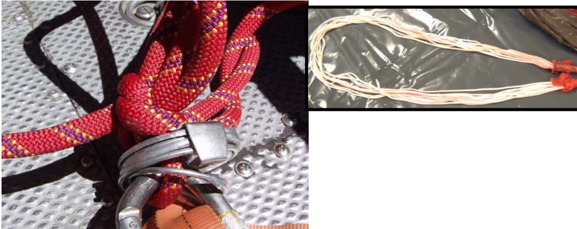
Figure 3 “While hoisting a seriously injured climber from the Cathedral Spires Gully the aircraft experienced a decay in rotor RPM with a resulting loss of heading control and altitude. As the crew worked to control the aircraft the hoist cable struck a tree and separated. The rescue corpsman and climber were retained on the belay line 20 .” The belay device in this scenario held a rescue load without failing the dynamic rope; note the stopper knot behind the device that spontaneously formed during the accident to prevent the corpsman and litter from hitting the ground and possibly bringing down the helicopter thereafter. The photo on the right shows the sheath stripped from core after being loaded with a stopper knot at the belay device.
