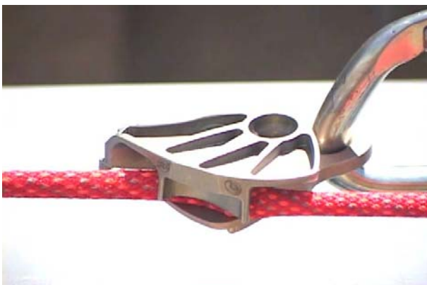
Figure 15: A static mode of failure for a device with tail tension; the rope is released from the belay device through the small gap shown.
