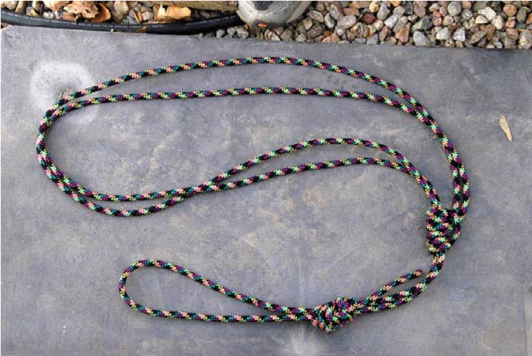
Figure 9: Drops were conducted on Purcell prussiks using two different loads
