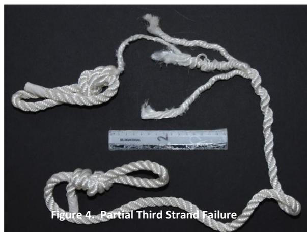
Figure 4. Partial Third Strand Failure
