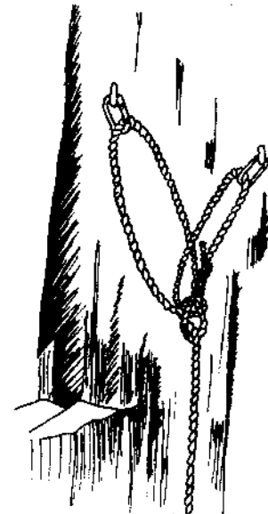
French bowline is used with two offsetting rig points. The knot will equilibrate tension on both points. Notice overhand backup shown.
