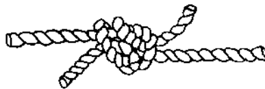
Pull the two overhand knots together to complete your Fisherman's knot.
