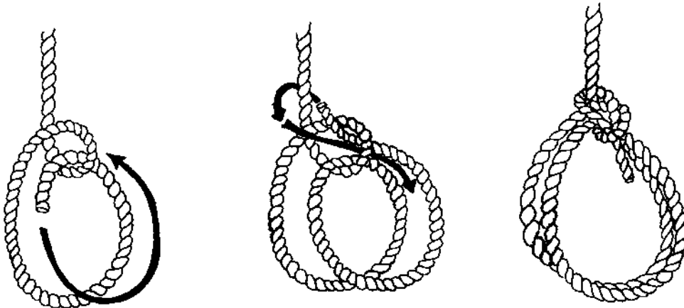
French Bowline or self equilizing bowline. Sometimes referred to as a double bowline, but I don't believe that is a correct nomenclature.
