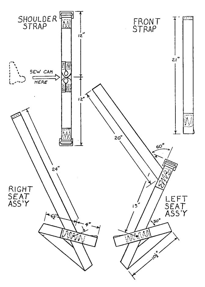
The RIGHT SEAT assembly clips into the seat biner, forms a leg loop, and attaches to the other half of the seat by a buckle in the rear. Do not make the leg loops too tight. The dimensions shown fit me, they may not fit you. Since the buckle need never come completely apart, you're advised to fold the end of the webbing to form a knob, as in the foot cam.
