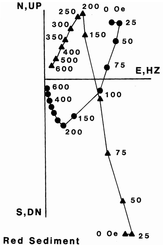
**Figure 4.** Demagnetization diagram showing primary and secondary components of magnetization. Dots indicate magnetic declination plotted in N, E, S (north, east, south) coordinates. Triangles represent magnetic inclination plotted in UP, DN, HZ (up, down, horizontal) coordinates. Numbers show alternating field demagnetization intensity in Oersteds (Oe). Note that the normal secondary component is removed by 200 Oe demagnetization step.
