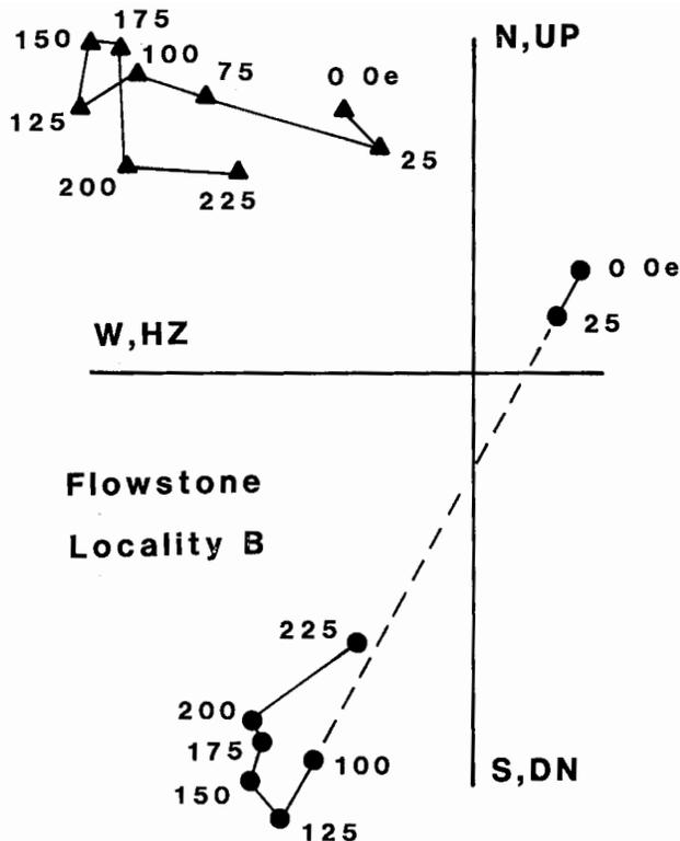
**Figure 5. Demagnetization diagram of flowstone sample from locality B. See figure 4 caption for plotting conventions. Secondary components appear to be removed by 125 Oe demagnetization. While the characteristic direction is not well-defined, all measurements between 200 and 350 Oe shows a southwest (S, W) and negative (UP) direction, a reversed magnetization.**
