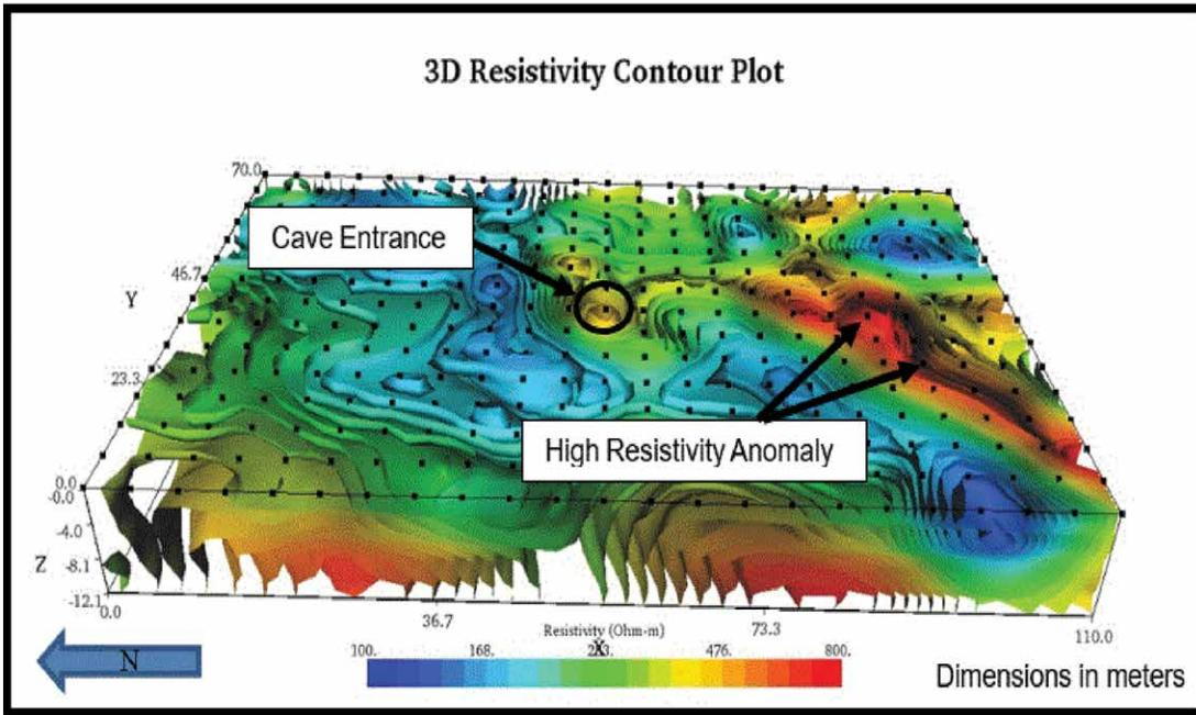
Figure 4. Resistivity contours illustrate the Friesenhahn Cave area. Black dots represent electrode placements and are five meters apart.
