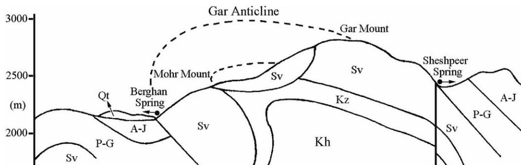
Figure 4. Geological cross section between Berghhan and Sheshpeer Springs, The legend is shown on Figure 3 (after Raeisi et al., 1993).
