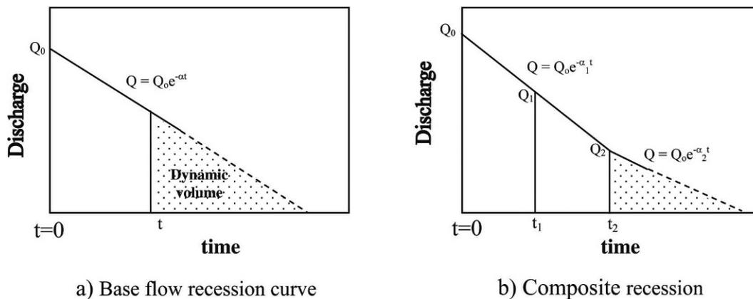
Figure 2. Schematic diagram of recession curves: a) base flow recession curve; b) composite recession curve.
