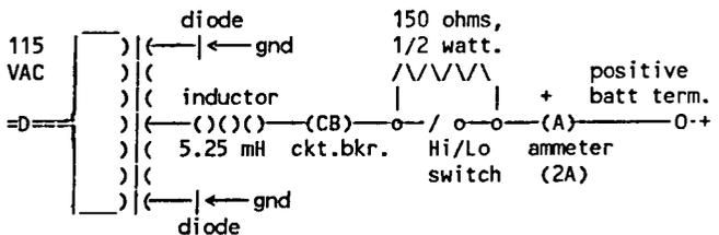
gnd = chassis ground, also negative battery terminal.
