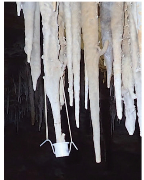
PVC Speleorake for retrieving broken material from pools
