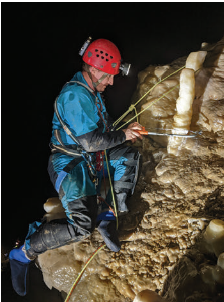
Greg Roemer-Baer (Expedition leader-CRF WEST) operating saw. It is rare to take complete speleothems for climate studies. Most studies can be accomplished with small cores taken from the speleothem—the portion containing the surface of the speleothem is often returned to the cave and used to plug the hole where the core was drilled.
