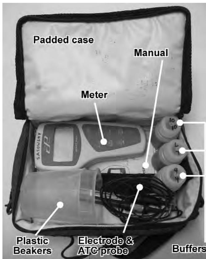
**Figure 2. Example of a kit for field pH measurement in karst settings.**
