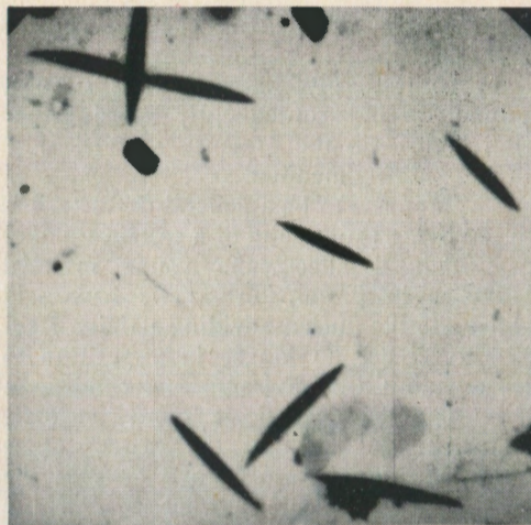
Figure 7 Elongated spindles from limonitic clay from St. Catherine Cave, Ariège, France. X5,000.
