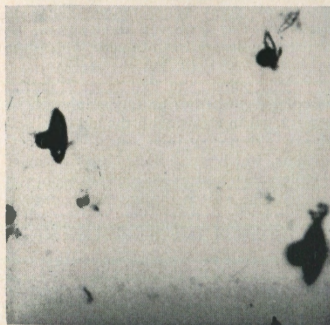
Figure 8 Budding spindles from limonitic clay from St. Catherine Cave. X5,000.
