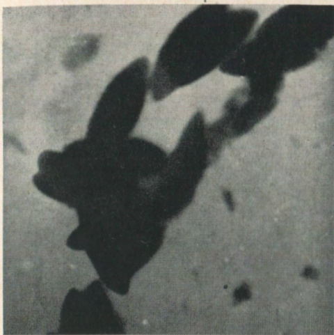
Figure 2 Needles of ferric hydroxide dilated by hydration. X9,500.
