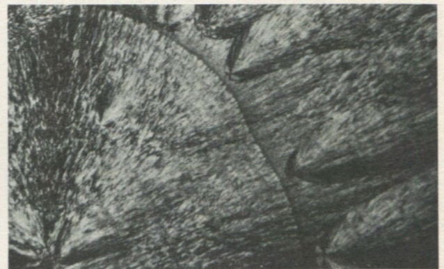
Fig. 5. Photomicrograph of a silica stalactite. Note the optically fibrous radial structure under crossed nicols.
