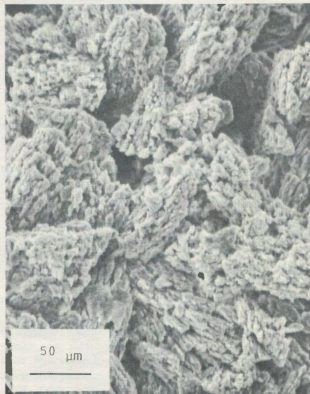
Fig. 10. Scanning electron micrograph of the surface of an appelite speleothem. Note that the crystal-like forms are random in orientation. However, 20 to 50 of these coalesce to form a group. A collection of groups form the typical botryoidal surface seen in hand specimens (Fig. 2).
