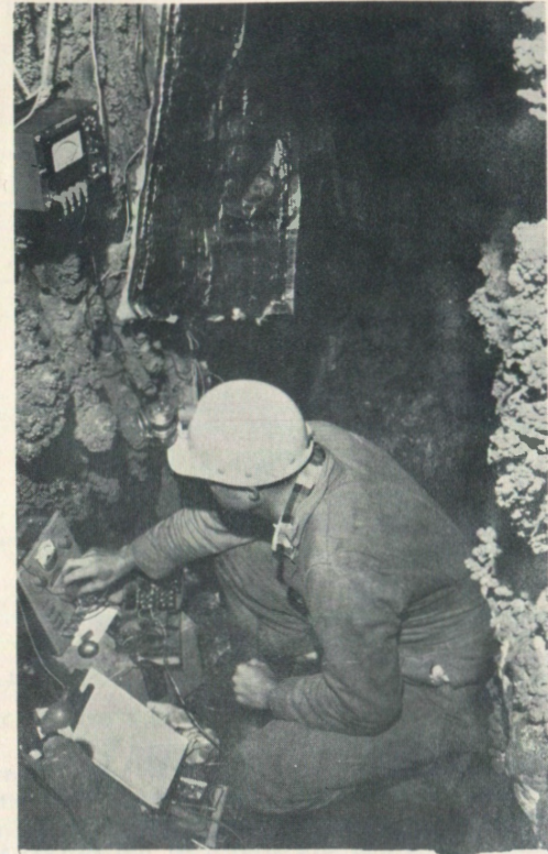
Figure 4. Temperature-readout meter above, and strain-readout meter below. The instrument station is under the sheet of insulation at top center. All photographs by Ellis Hedlund.
