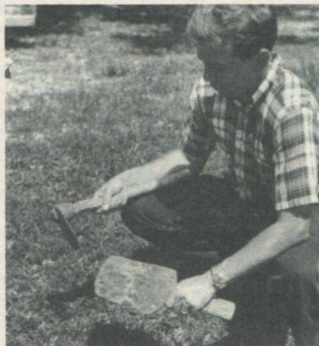
Figure 2. Iron mattock and wooden paddle, the basic saltpetre mining tools. Author's photo.
