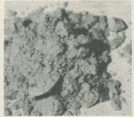
Figure 4. Crystalline materials obtained in the salt-peter process: (a) — (above, left) first appearance of arcanite crystals ( K_2SO_4 ); (b) — (above, right) first crystal crop — arcanite; (c) — (left) second crystal crop — arcanite and schoenite ( K_2SO_4 \cdot MgSO_4 \cdot 6H_2O ).
