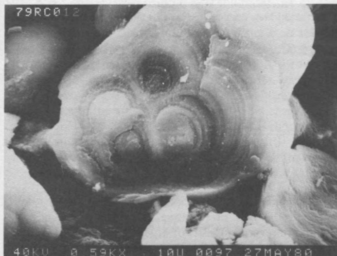
Figure 13. SEM image of cross section of manganese-rich nodule (79RC012) showing layered structure.
