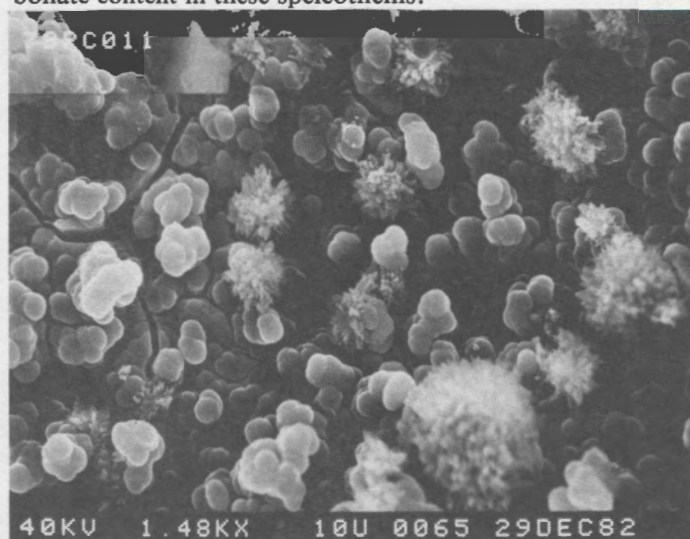
Fig. 10. SEM image of white stalactite 79RC011 showing nodular masses with interspersed 'flowers.' Image width 77\text{ }\mu\text{m} .
