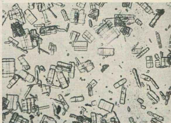
Figure 1 Photomicrograph of the peculiar type of gypsum described in this paper.
