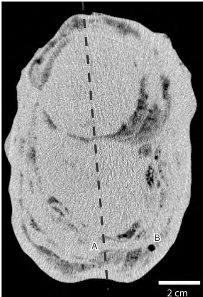
Figure 2. HRXCT slice through AH-M showing density variations. Higher densities are indicated by lighter gray scale values. Two sets of concentric growth bands are visible. The upper set was apparently deposited before subsidence of the speleothem. The lower set indicates the location of the new growth axis on the flanks of the previously deposited speleothem material. A plane that bisects both growth axes is easily determined (dashed line A). A large void, near B, may be filled with air or the water from which this speleothem precipitated.
