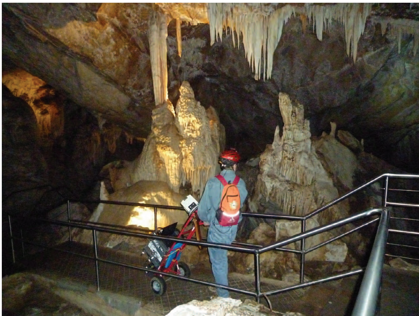
Figure 3. The Hannibal mapping cart in operation in Lucas Cave, Jenolan.
