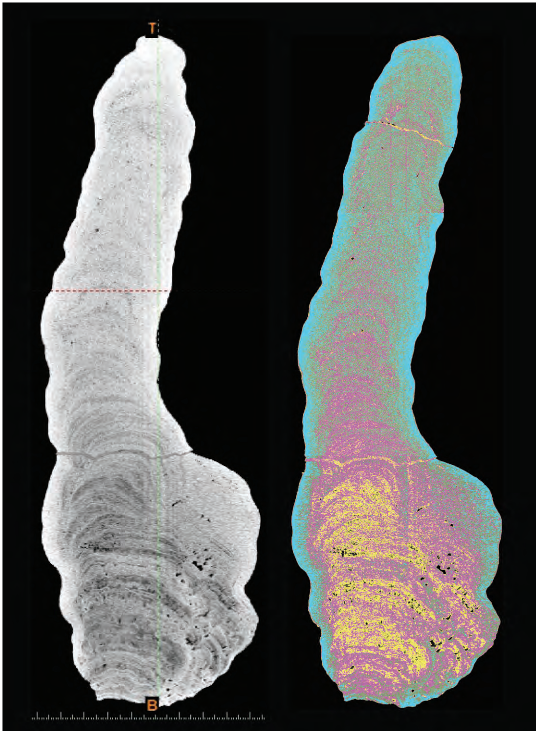
Figure 3. 2D image of section of the stalagmite Novella. On the left is the unprocessed radiograph of the stalagmite. On the right is the radiograph of the stalagmite with the different calculated density-ranges. Each color has been found to correspond to different crystalline textures recognized in the petrographic study. Black is -1024-226 Hounsfield units, lowest density values, air-filled porosity; yellow is 227-776 HU, low density values, dendritic crystalline texture; fuchsia is 777-1176 HU, medium density values, closed dendritic crystalline texture; green is 1177-1576 HU, high-density values, columnar crystalline texture; and blue is 1577-3071 HU, highest density values, micritic crystalline texture. The colors are superimposed here, with those representing the lowest densities on top.
