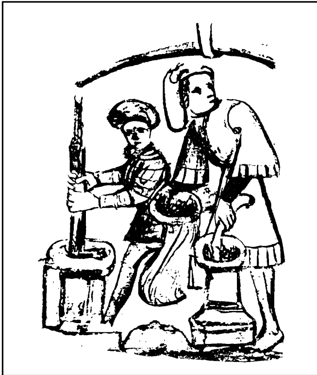
Figure 1. Earliest known illustration of gunpowder manufacture, circa 1350, cited from the Codex Germanicus #600 and published in Oscar Guttman, Monumenta Pulveris Pyrii (privately printed, 270 copies, 1906). Accompanying text, translated: "If thou wouldst make a simple powder of three parts, only then take four pounds of saltpeter, which must be good and well refined and one pound of sulfur and one of charcoal and pound it in good wine in which camphor has been boiled and dry it in the sun. If no camphor is in it, the powder easily falls to dust but the camphor holds all together and is powerful and quick in all powder into which it be put." (Illustration courtesy of Hagley Museum and Library, Wilmington, Delaware).
